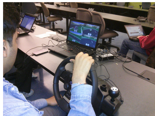
Fig. 10: A human controlling a vehicle within TORCS environment to test the fuzzy logic ACC.
