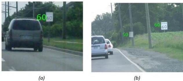
Fig. 8: (a) shows the successfully recognized speed sign, and (b) shows an image with a false positive recognition.
