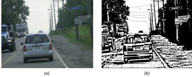
Fig. 5: (a) shows the original image and (b) shows the locally thresholded image with the subtracted green channel
